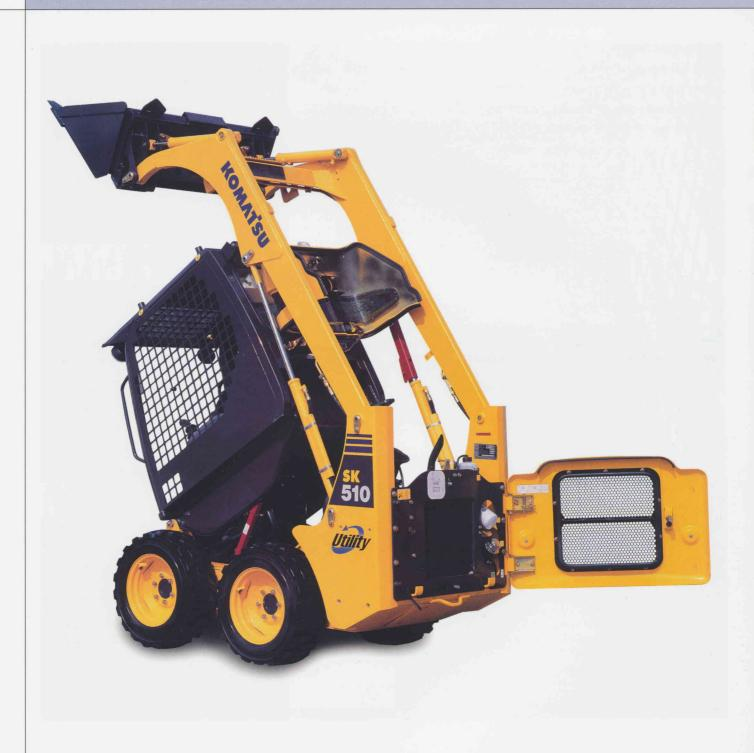
The routine maintenance and checks can be performed by simply opening the rear bonnet. In addition, the opening of the back allows the user to access and clean the radiators (which can be inclined). Then, for special service operations, the tilting cab offers complete access to the transmission and to the main components of the hydraulic system.
